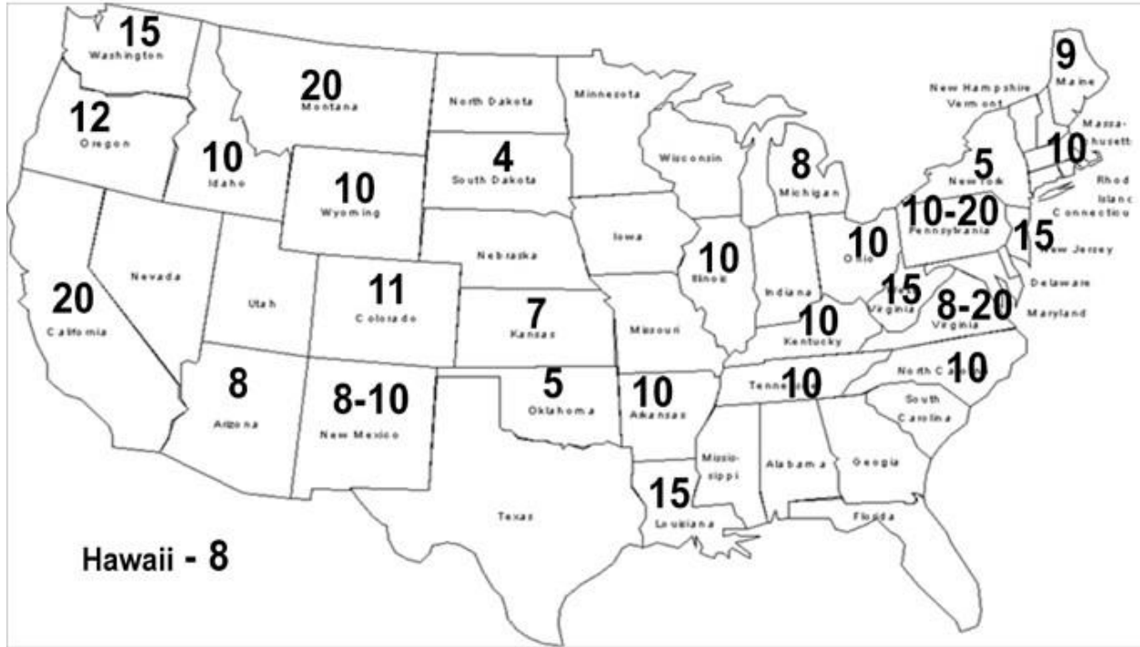
Figure 2: DOT reported preliminary engineering cost as a percentage of construction cost (Hollar 2011)
